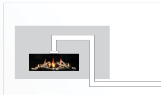
End of line flush horizontal Power Vent system shown in a negative vent run
